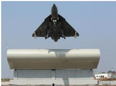
The LCA Navy aircraft is being developed to incorporate a drooped nose for better over-the-nose vision and to feature strengthened fuselage structure, redesigned landing gear to cater to higher loads, arrestor hook for deck recovery, leading edge vortex control (LEVCON) surface to reduce approach speed, fuel dump for emergency deck recovery and operational capability on an aircraft carrier by way of ski-jump take-off.
