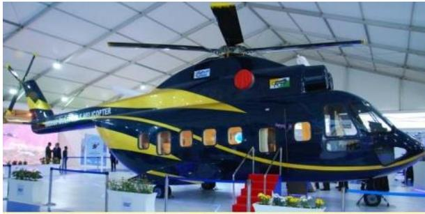
The IMRH will be co-designed and co-produced as a medium lift helicopter in the 10 to 12 tonne class to meet the requirement of the Indian Army and the Indian Air Force. The helicopter will be powered by twin engines and will feature blade folding option for ship deck operations. The IMRH will support air assault, air transport, combat logistics, combat search and rescue and casualty evacuation operations. We have yet to select a technological partner for this project.
