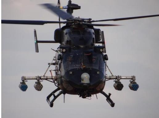
The ALH Mk IV Rudra is a weaponised platform designed for attack mode with the capability to carry external stores. The ALH Mk IV is equipped with an integrated architecture display system with multi-function displays. The helicopter can be fitted with four rocket pods or two air-to-air missiles as well as a 20 millimetres nose-mounted turret gun. We delivered the first Rudra helicopter in 2013.
