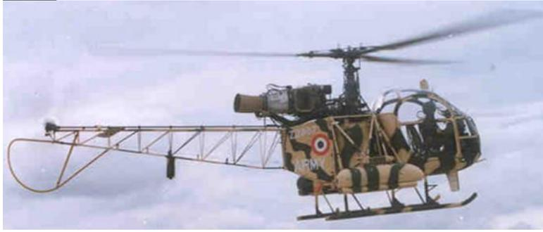
The Lancer is a weaponised version of the Cheetah helicopter as modified by us. The Lancer is a light attack helicopter which is equipped with two jettisonable combination gun-cum-rocket pods and a gun sight for accurate aiming and firing by the pilot. The Lancer is optimised for anti-insurgency operations, particularly in mountains and jungles.
