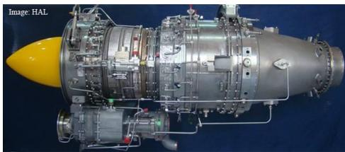
Indigenous design and development of a 25 kN thrust class turbofan engine has been taken up for use in basic military trainer aircraft/business jets. We believe that the development effort through this medium sized turbofan engine constitute an important step toward helping enable the country to achieve self-reliance in the design of this class of aircraft turbofan engines.
