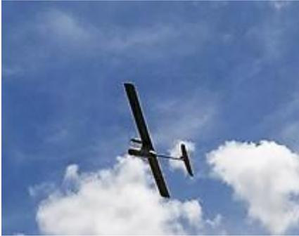
The indigenous design and development of mini UAV of the eight kilograms class is to meet the emerging requirements of military, para-military, police and civil sectors. It consists of fully composite structure, robust, rugged and man-portable system. It can be used for surveillance, reconnaissance and target tracking mission. We have made product demonstrations to prospective customers.
