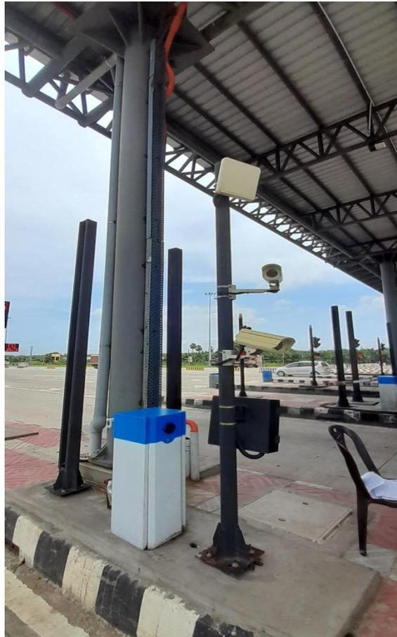
**Figure 9-2 RFID ETC Transceiver installed on pole**
