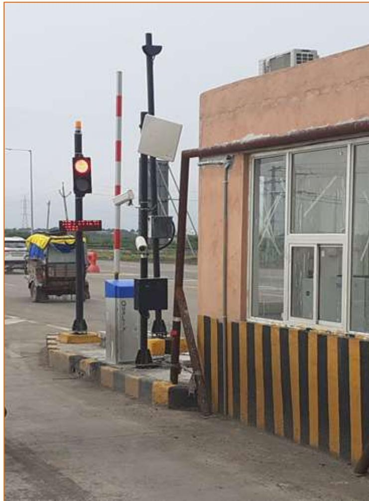
Figure 8-2 RFID Scanner located on pole
